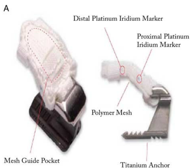
FIGURE 1. An illustration depicting (A) the Barricaid device and (B) the device implanted. This device has a titanium anchor that is placed into the lower vertebral body using tamp and mallet. The mesh polymer expands across the entirety of the intervertebral space, overlying the residual physiological nucleus pulposus. Two platinum-iridium markers within the polymer mesh allow visualization on plain films. full color online
