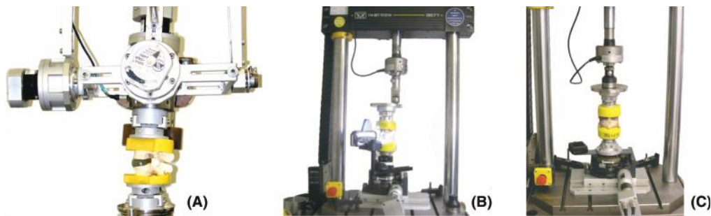
Figure 1. (A) Spine segment fixed into the spine-tester for the flexibility test. (B) Cyclic loading setup showing the rotation base with the mounted specimen and the video camera, which records the extrusion. (C) Setup for height measurement.
